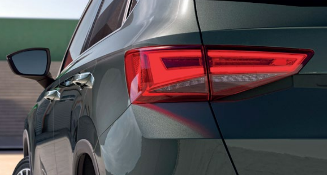
LED tail lamps with dynamic blinker
